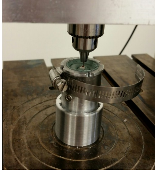
Figure 6.2. Custom-designed and fabricated fixture for biomechanical testing. Photograph was obtained just prior to wire pull-out.
